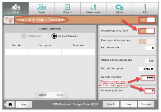
9. On the left side of the screen, enter the Barcode and Description information from Table 5 below into the Optical Detection table.
