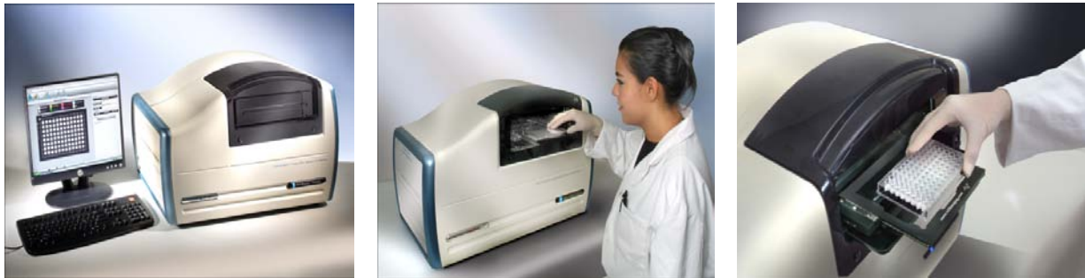
Figure 8. (1) Biocode 1000A System, (2, 3) Manual loading of Microplate and Automated Loading Tray
